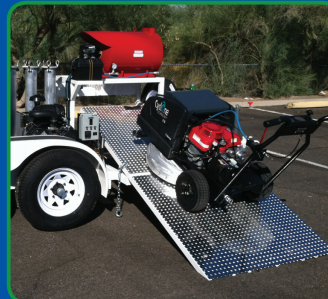
Pivoting ramp allows winch easy loading and unloading of the CY210 walk-behind.
